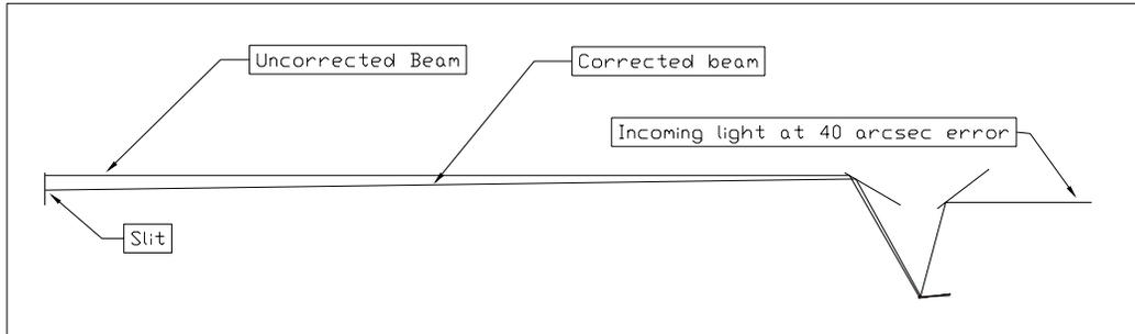
Figure 7. Exaggerated Corrected and Uncorrected Lightpaths. The tip/tilt mirror is rotated clockwise slightly to compensate for the 40 arcsecond downward error.
