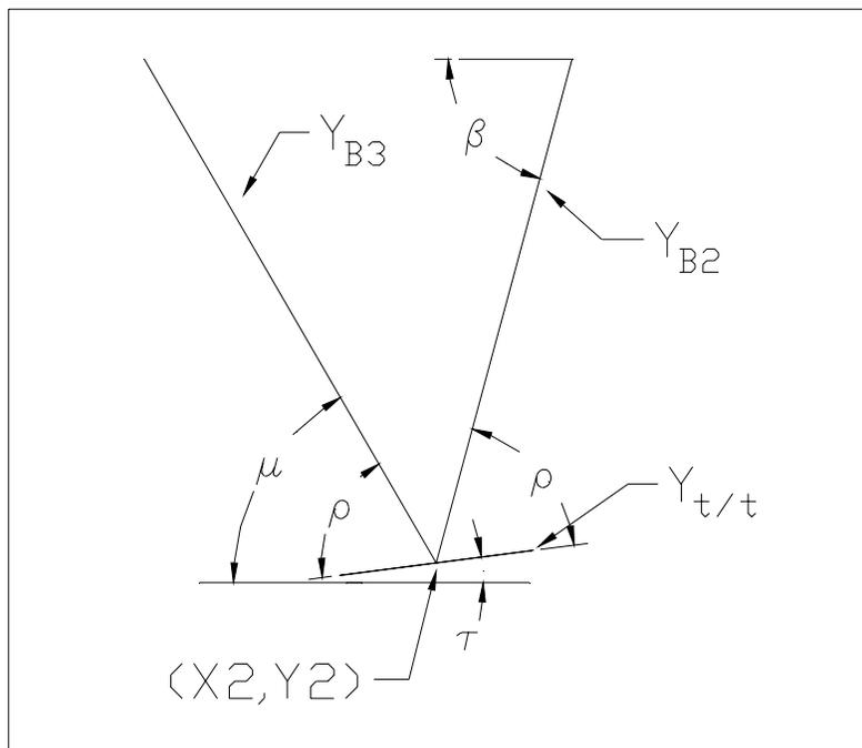
Figure 10. Geometry for Tip/Tilt Mirror and Beam Angles.
