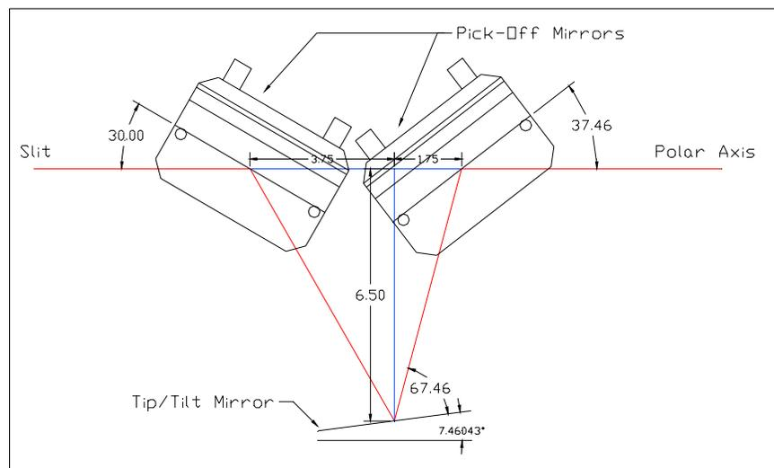
Figure 5. Mirror Layout. Mirror layout on optical table and angles with respect to the ideal light path.
