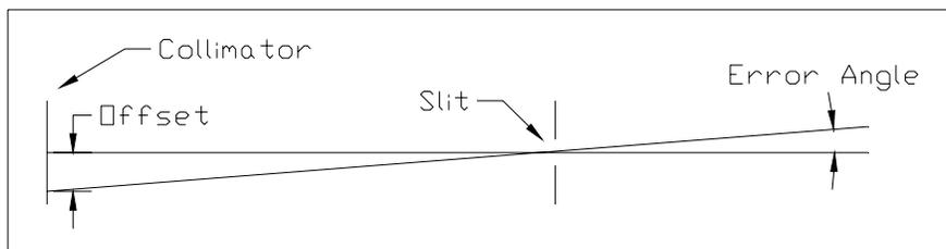
Figure 12. Error Angle ( $\sigma$ ) Vs. Collimator Offset.
