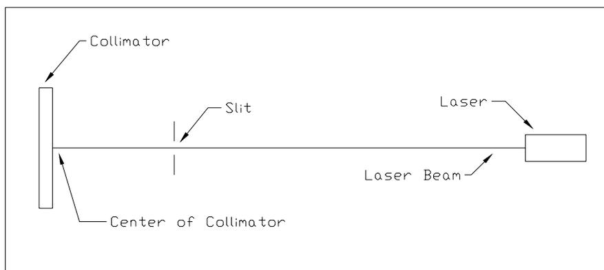
Figure 14. Alignment Laser. Laser simulates optical axis by aligning it to pass through two known points of the optical axis.
