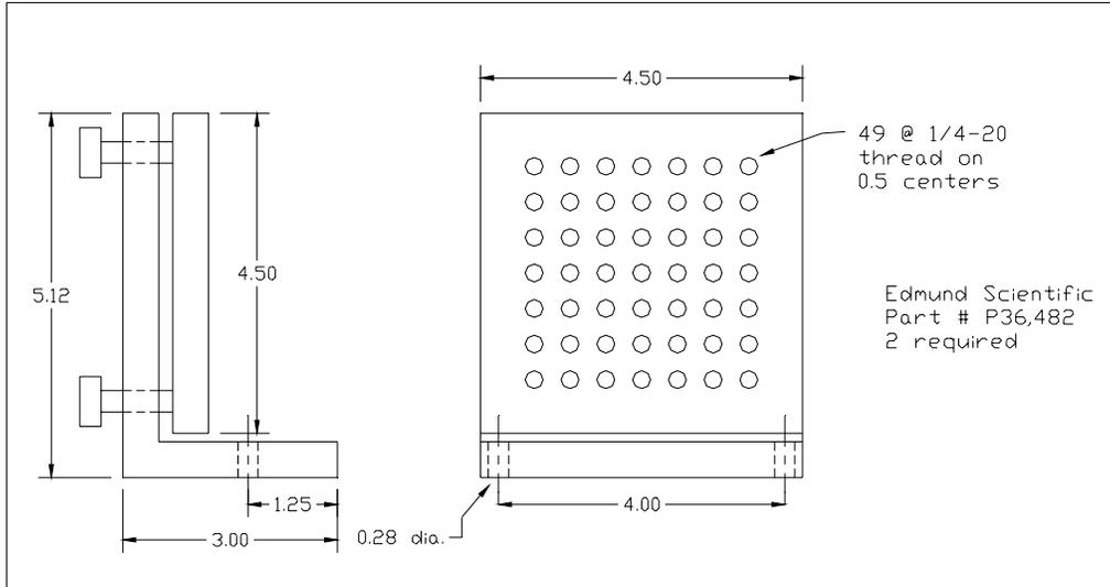
Figure 6. Pick-Off Mirror Mount. Mount is on a kinematic stage with 8 degrees of adjustability.
