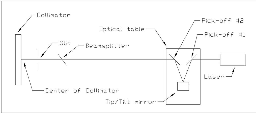
Figure 15. Optical Table Alignment Setup. The optical table is aligned by adjusting the pick-off mirrors such that the laser passes through the slit and the center of the collimator.
