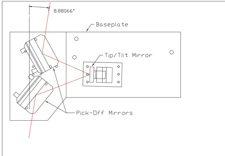
Figure 4. Optical Table Assembly. The dashed line represents the light path of incoming starlight. This light is picked off with the first mirror, reflected off the tip/tilt mirror for corrections and inserted back into the original light path before continuing on its slightly modified path to the slit.
