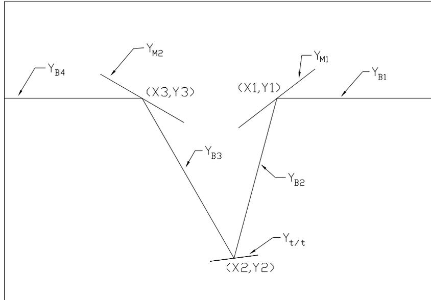
Figure 8. Layout of Mirror Surface Lines and Lightpath Segments. The lines are defined in rectangular coordinates of the form  $Y(X)$ .
