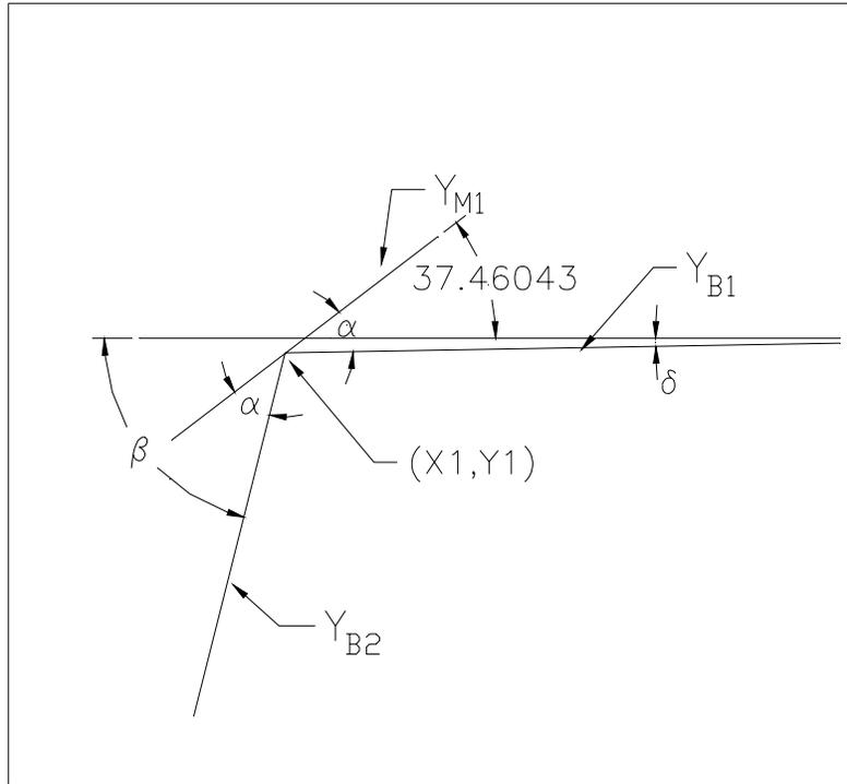
Figure 9. Mirror 1 Reflectance Angles. Angles are in terms of incoming starlight angle  $\delta$ .
